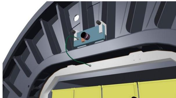
**Figure 5: Sensor Package as an Externally-Mounted Hosted Payload**
