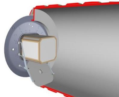
**Figure 9: HatchBasket Installed in Cargo Vehicle Hatchway**
