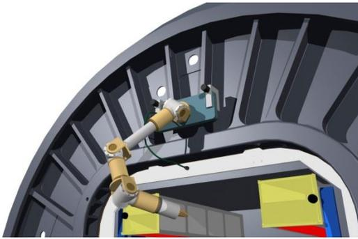
**Figure 6: Robotic Manipulator as an Externally-Mounted Hosted Payload**
