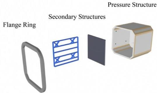
**Figure 1: HatchBasket Components**
